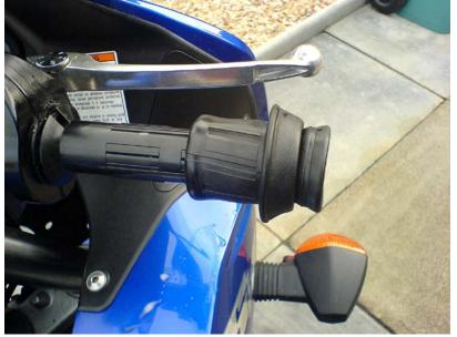
Once removed, the bars will require all old adhesive to be cleaned off.
