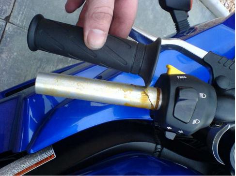
Left grip removed intact and showing adhesive residue on bars. Fine sandpaper can be used to aid the removal of old adhesive from the bars. Clean with meths afterwards to ensure a clean surface for the new grip glue.
