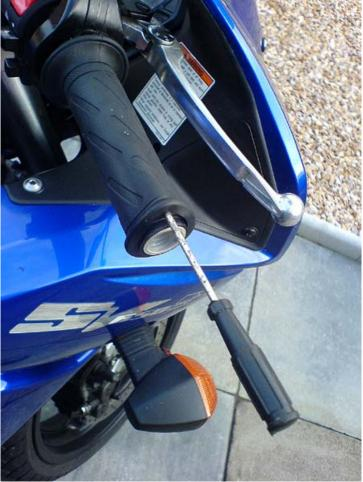
The use of this technique will turn the screwdriver between the bars (or throttle tube) and the grip, removing the adhesive all around the diameter. The grip can then be pulled off in the case of the left hand side, or rolled back from the throttle tube in the case of the right hand grip.
