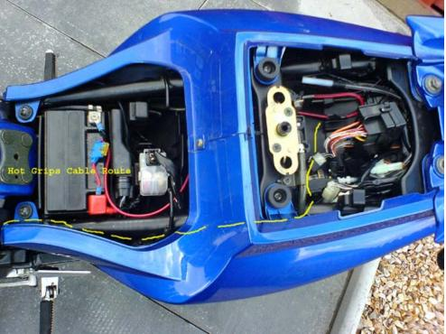
The fuse box is on the right (under the pillion seat or cowl) and is identified by the mass of wires entering its lower edge. It is shown here after being released. Simply lift the fuse box upwards, since it hooks onto a tab at either side.
