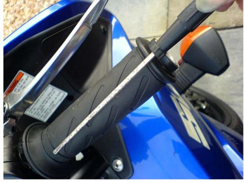
Insert the screwdriver underneath the length of the grip and turn the handle as you go.
