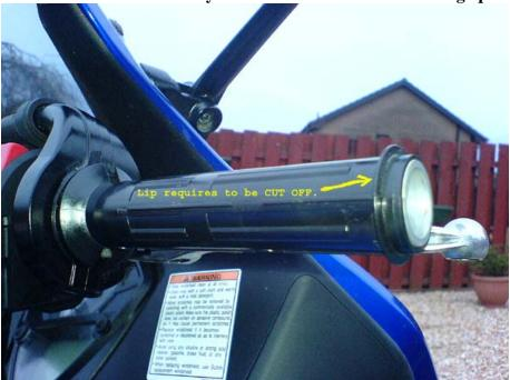
The bike in the picture needed a lip on the throttle tube to be cut off in order to slide the new grip on. Careful use of a sharp craft knife was all that was needed. You can also see a tapered end on the inside – more of this later.... Here are the original grips after removal with the Hot Grips before fitting.
