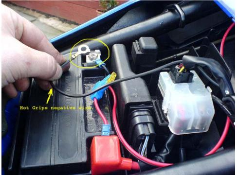
Note that the (heavy) red & black cable with fuse holder is an extra on this bike.
