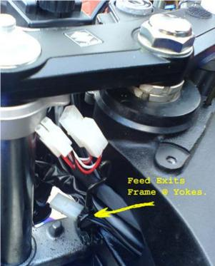
From the front of the bike, we see the power feed in place but not snapped together.
