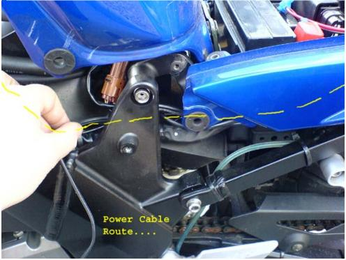
Note the main cable loom to which the power lead can be tie wrapped.
