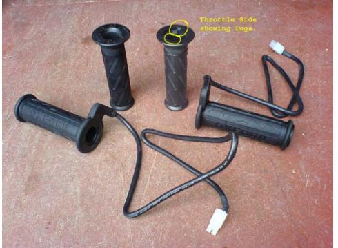
The new "Hot Grips" are slid into place (or shoved hard in some cases) as per the manufacturers guide. It IS worthwhile checking their operation as well as position prior to glueing them into place. Make sure that the heater cable exit from each grip does not hinder any controls at all handlebar positions.
