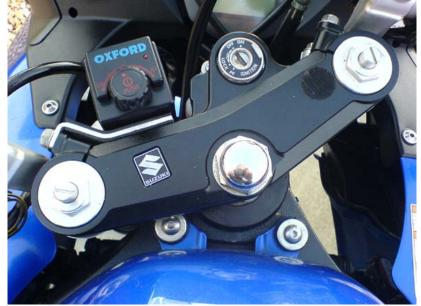
2) With the easy bit done, we need to turn attention to the installation of the power feed cable. It would be too easy to leave the grips switched on with the bike parked up, or for kids to switch them on draining the battery and leaving you stranded. With this in mind, we really want to use a suitably rated power feed that is only "on" when the ignition key is turned on. Fortunately enough, the "pointy" SV has a couple of spare contacts in the fuse box which can be tapped for this purpose.
