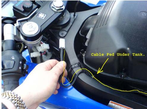
Once at the front of the air box, you will find a cable passage in the frame to pass the feed through. This will bring you to the headstock, where your controller cable will be able to meet its matching connector.
