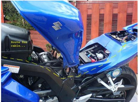
The proposed cable route has been added in yellow. Please note that when routing the cable, care should be taken to cable tie it against the main cable loom to prevent any chaffing against edges of the frame.
