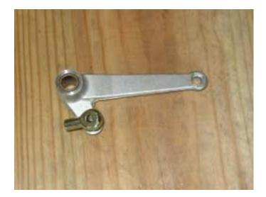
I purchased a stainless 5/16" machine bolt (figuring that this would be least likely to rust) with a tapered head and an acorn nut to match. The bolt fits into the drilled out hole and sits recessed in the hole because of the tapered head. The head is facing the bike and will not have any interference with other moving parts.
