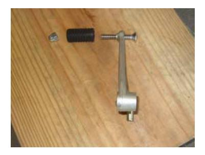
Taking the rubber off of the original and reinserted on the threads of the bolt, it is held in place with the acorn nut. The acorn nut is rounded, so I don't think it would cause too much friction. Here is what the final product looks like:
