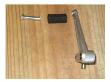
I drilled out the spot where the original was welded with a 5/16" drill bit. I used a punch to mark the center of the hole so that the drill bit doesn't wander. I also widened the hole with a 3/8" drill bit, but only at a depth of less than approximately \(^1/4\)" (you will see why next).
